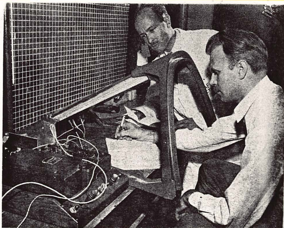
TESTING DISTORTION. This Avro CF-100 windscreen is being tested for optical distortion by E. G. Revette, an Avro inspector. With him is G. D. Jones, RCAF inspector of aircraft. The distortion is being measured by the photo-grid system.
