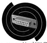
D Sub-miniature rack/panel type; steel shell protected; all 5-amps. 15 to 50 contacts; flash. 1700v dc: junction shells, locking means; floating mounting holes; also hermetic seals.
