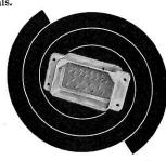
Miniature rack & panel type; shell protected; 13 available insert arrangements; 5-amp, 10amp and miniature coaxials; split shell.
