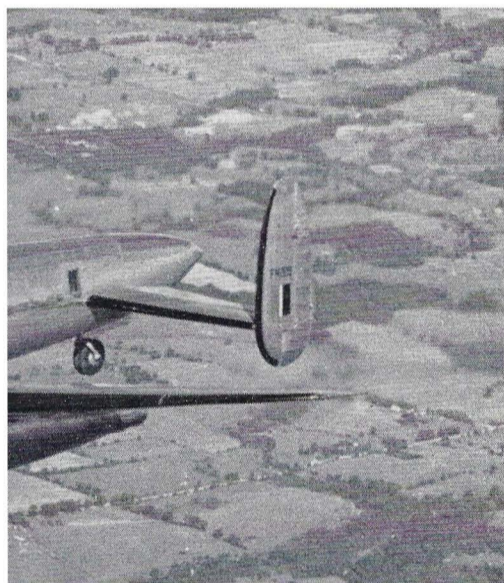
The Orenda was first flight-tested in this converted Lancaster using two conventional piston engines inboard, two Orendas outboard.
