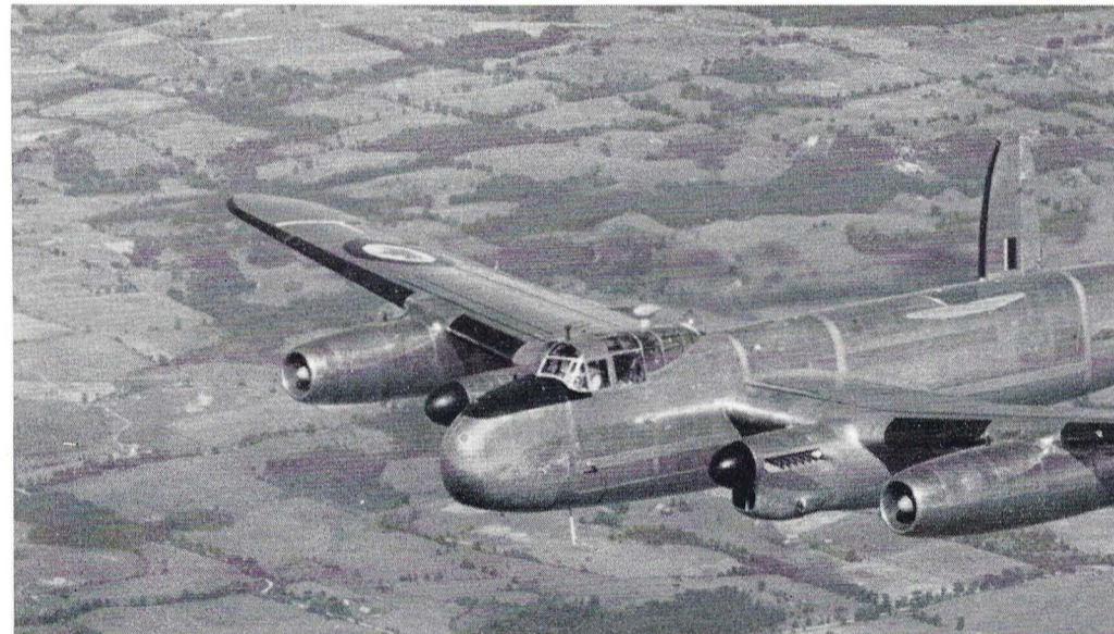
The Orenda was first flight-tested in this converted Lancaster using two conventional piston engines inboard, two Orendas outboard.
