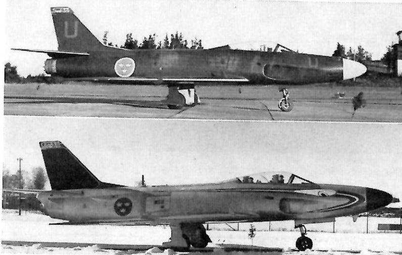
SAAB-32 LANSEN: A new version of the Saab-32 Lansen, two-seat all-weather aircraft, the J-32B (above), has been specially developed for all-weather and night interception. It differs from A 32A version by having more powerful engine with enlarged afterburner. Below: another new Lansen variant, the Saab-32C photo-reconnaissance version, which is fitted with the most modern photo equipment and has provisions for several different equipment alternatives.
