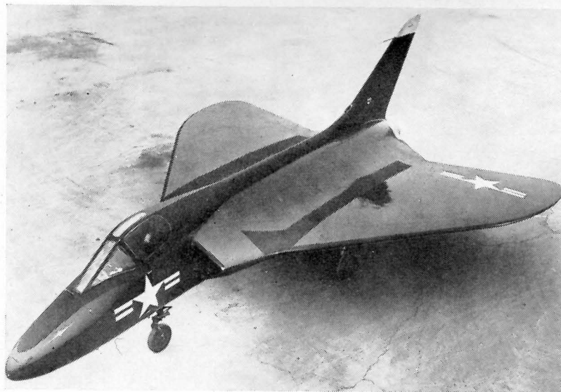
SPECIALIST: Designed for the USN especially for interception work, the Douglas XF4D made its first flight early this year. Powered by a Westinghouse XJ-40 turbo-jet of 7,500 pounds thrust, the XF4D is intended for catapult take-offs and fast climbs. The aircraft features an elliptical form of the delta wing and a high narrow vertical tail. Cockpit bears strong resemblance to design used on the Douglas A2D.
