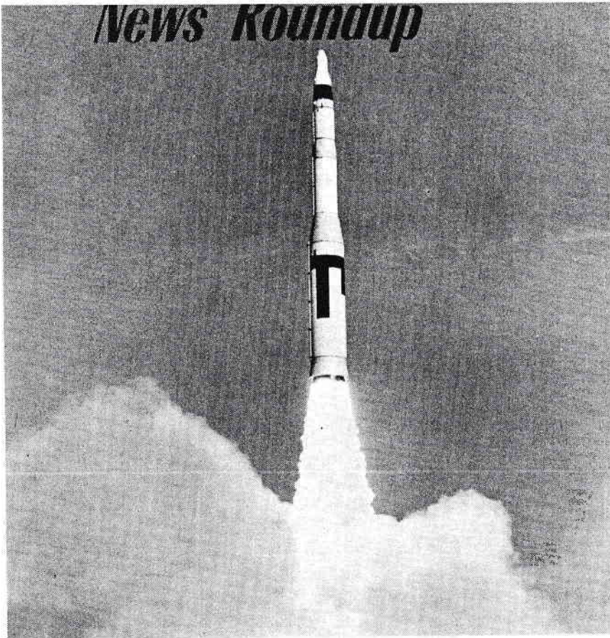
THE SOLID-FUELED BOEING MINUTEMAN , the USAF's newest ICBM, is shown being launched for the first time. Test firing was pronounced successful when all three stages fired and nose cone landed in target area. Minuteman missiles will be located in underground silos and on roaming trains.
