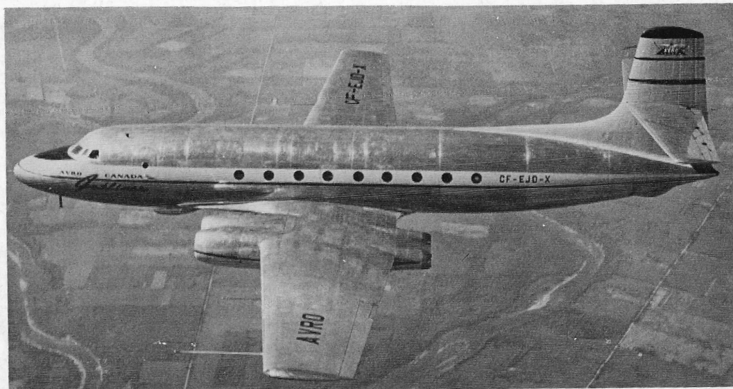
The Avro Canada C-102 Jetliner - the first jet-powered airliner to fly in North America, preceded in this respect only by the DH Comet I in England. This rarely seen Avro photo is reproduced courtesy of Neil Christenson.
