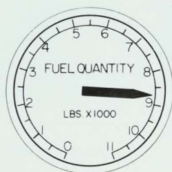
Figure 19. Fuel Quantity Meter
