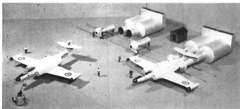
JET MUFFLERS: These strange new shapes will begin to appear along Avro Aircraft Limited's flight line starting in May. They will be the first of six twin units for muffling the engines of the CF-100 during engine run-ups. Each unit is composed of a steel baffle tank about 26 feet long and 12 feet in diameter, with an exhaust pointing upwards. On the front are tubes to take the special mobile adapters which connect to the CF-100 tail pipes by rubber seals.
