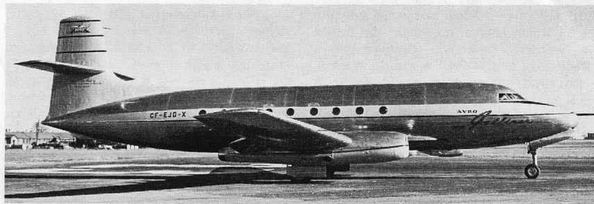
(Above and below) The Avro Canada C.102 was the world's second commercial transport designed from the outset for turbojet power to commence its flight test programme.
