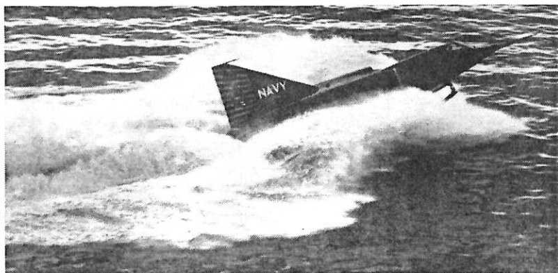
SEA-DART: The world's first delta wing seaplane, the XF2Y-1 "Sea-Dart", is shown during taxi tests and (lower right) beached. Made for the USN by Consolidated Vultee, the Sea-Dart incorporates retractable hydro skis and is powered by two unidentified Westinghouse turbojets, presumably J-34's of some 3,400 lbs. th. each. Navy thinks this aircraft will equal performance of land-based machines.
