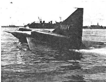
SEA-DART: The world's first delta wing seaplane, the XF2Y-1 "Sea-Dart", is shown during taxi tests and (lower right) beached. Made for the USN by Consolidated Vultee, the Sea-Dart incorporates retractable hydro skis and is powered by two unidentified Westinghouse turbojets, presumably J-34's of some 3,400 lbs. th. each. Navy thinks this aircraft will equal performance of land-based machines.
