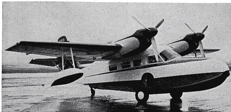
SUPER WIDGEON with Lycoming GO 480-BIB — 270-hp engines and Hartzell 3-bladed props is one of the 6 bought in France and converted by McKinnon-Hickman Co., Portland, Ore. It's claimed it can do 1750 fpm climb with full gross of 5,500 lbs; take off in 19 secs. at 6,300-ft. altitude and 100° (Lake Tahoe); and a claim of 1,000 mile range at 70% power giving 170 mph. It's completely revamped inside. Sells at $75,000 by Vancouver Aircraft Sales Ltd.
