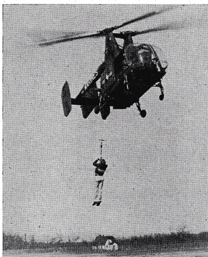
LATEST 'COPTER. An all-purpose Kaman HOK-1s gets a workout from the U. S. Marine Corps, which placed the intermeshing rotor craft in service recently. Power plants are 600 hp Pratt & Whitney Wasp engines.
