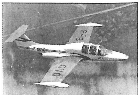
Below, the Morane-Saulnier MS-760 Paris, a four-place liaison version of the MS-755 Fleuret. The Fleuret was designed as a jet fighter trainer.
