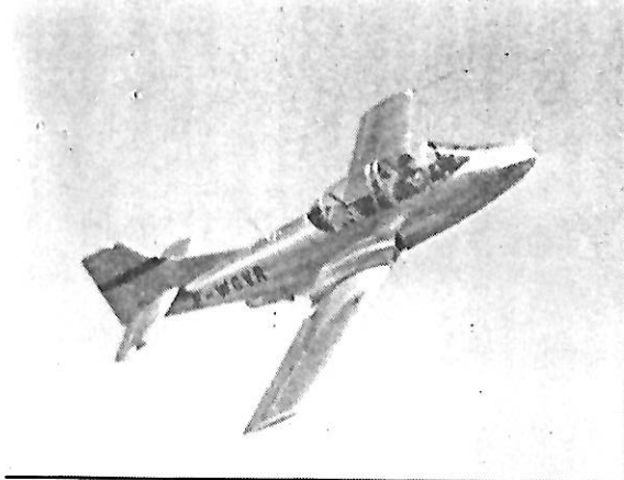
Above is the tandem SIPA 300 Primi-jet, while below is the side-by-side SIPA 200 Minijet, both French-designed and built for primary training.
