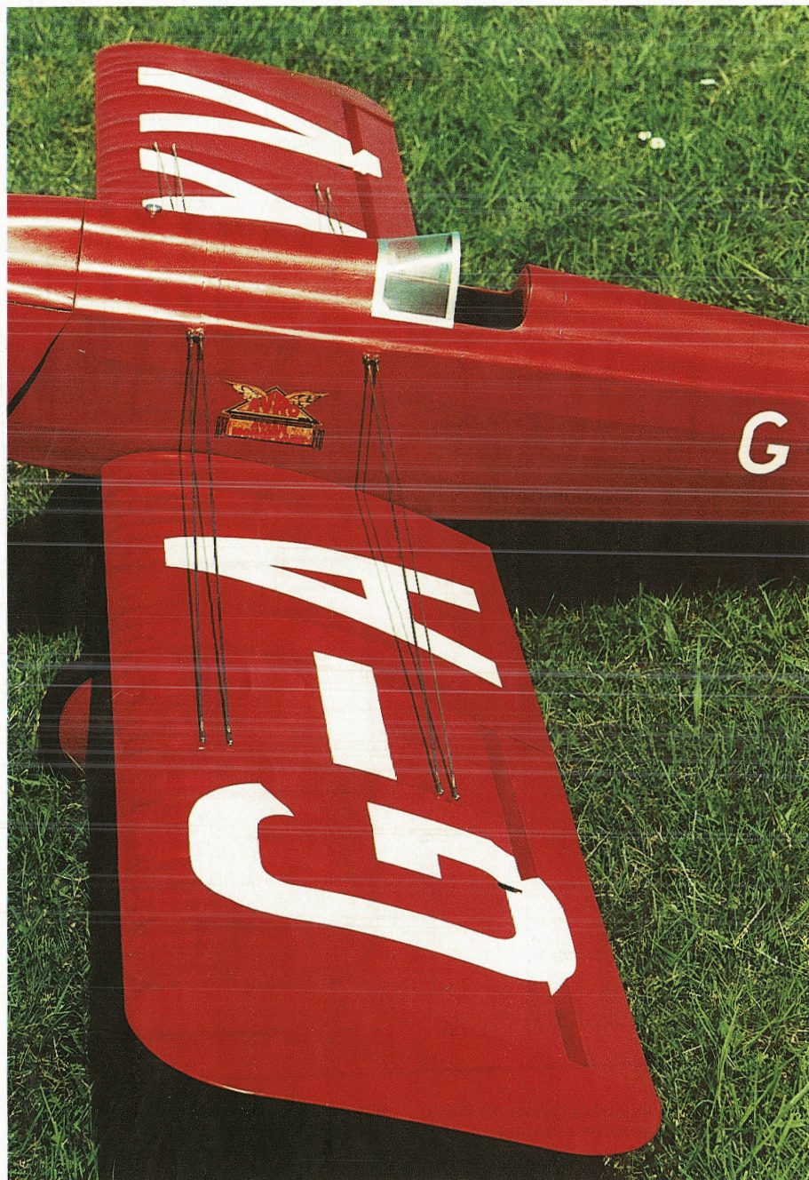
Wing registration lettering was hand-painted using card templates to mark position of characters, outlining with drafting pen then infilling by soft brush. Bracing wires are functional and should not be ignored.
