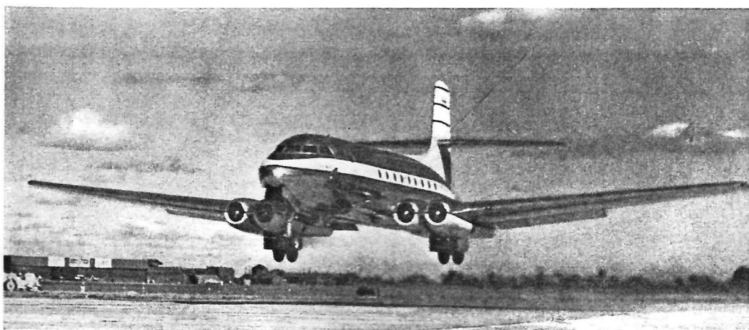
Fig. 2 : The "Jetliner" during the landing approach. Two Rolls-Royce "Derwent" gas turbines are paired in twin nacelles which also house the main landing gear.
