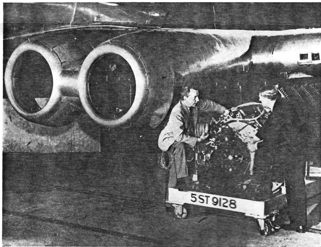
Fig. 8: Small distance above ground facilitates engine servicing.
