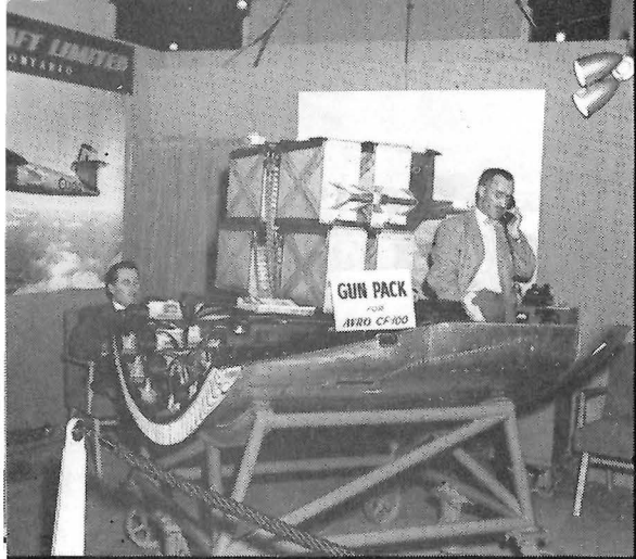
Above, left, Avro Aircraft had on display the CF-100's gun pack, complete with six .50 machine guns and ammunition cans. Avro Aircraft also showed a static test rig representing complete electrical system of the CF-100/4. At right is the Canadian Flight Equipment exhibit featuring the Martin-Baker Mk. CF-2 automatic ejection seat as made in Canada under license by CFE.
