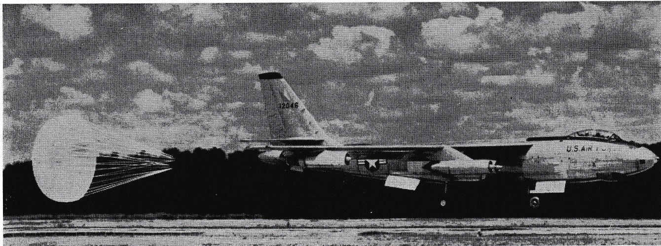
B-47 landing with its drag 'chute will soon be a familiar sight to Canadians living in Toronto, Montreal and Ottawa. This will be used as the flying test bed for Orenda's PS-13 engine which will be slung in a pod down on the side of the rear fuselage.
