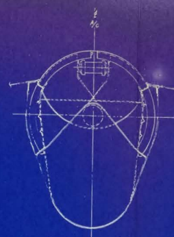
VIEW LOOKING AFT SHOWING PARACHUTE DOOR & BOX SCALE 1/4
