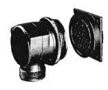
K Light weight, aircraft type connector ideal for many instruments. Connects and disconnects manually. Is held together by Acme thread coupling ring. Made in 7 shell types in 8 different diameters and more than 190 insert arrangements.
