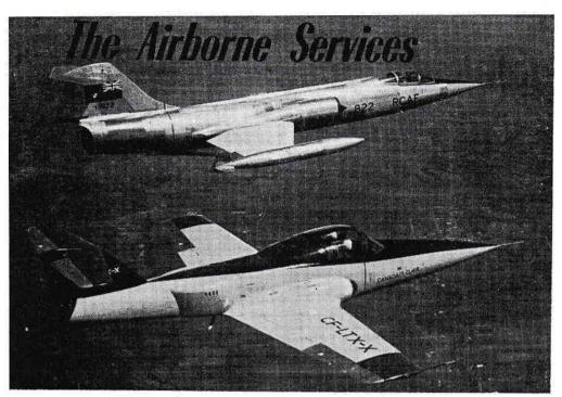
LIKE TWO CYRANO DE BERGERACS comparing noses, a Canadair-built CF-104 and the prototype Canadair CL-41R systems trainer fly side by side. The CL-41R carries the full range of NASARR systems for CF-104 and F-104G aircraft and is based on CL-41A pilot trainer, which RCAF has ordered.
