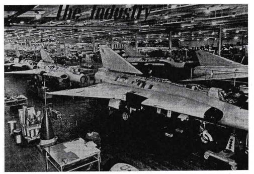
THE DRAGONS' LAIR is this large assembly operated by Saab Aircraft Co. in Sweden, where the Saab 35 Draken all-weather fighter is in quantity production for the Royal Swedish Air Force. Latest version is the S35B reconnaissance type, powered by the R-R RB.146 (17,000 lb./th. with reheat).
