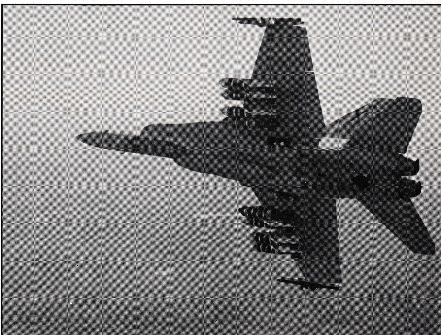
A CF-18 undergoing trials before acceptance by the Canadian Armed Forces. Contrast this cluttered, drag-inducing airframe with that of the Arrow, with its weapons pack retracted. This aircraft, now in service with Canadian squadrons, has a combat ceiling of 50,000 feet, and a maximum speed rating of Mach 1.8. This performance was matched or exceeded by the Mark I Arrow 30 years ago. The projected top speed of the Mark II, which never flew, was in excess of Mach 2. (Canadian Forces)
