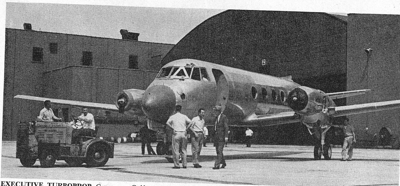
EXECUTIVE TURBOPROP Grumman Gulfstream is nearing completion at the Bethpage, Long Island plant. Plane heralds Grumman's re-entry into the business flying market. Due to fly this month, it is powered by Rolls-Royce Dart engines.
