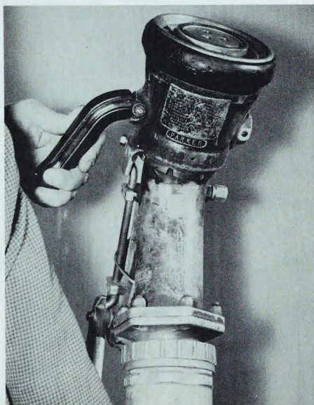
(B) REFUEL CONNECTOR ON THE TENDER
