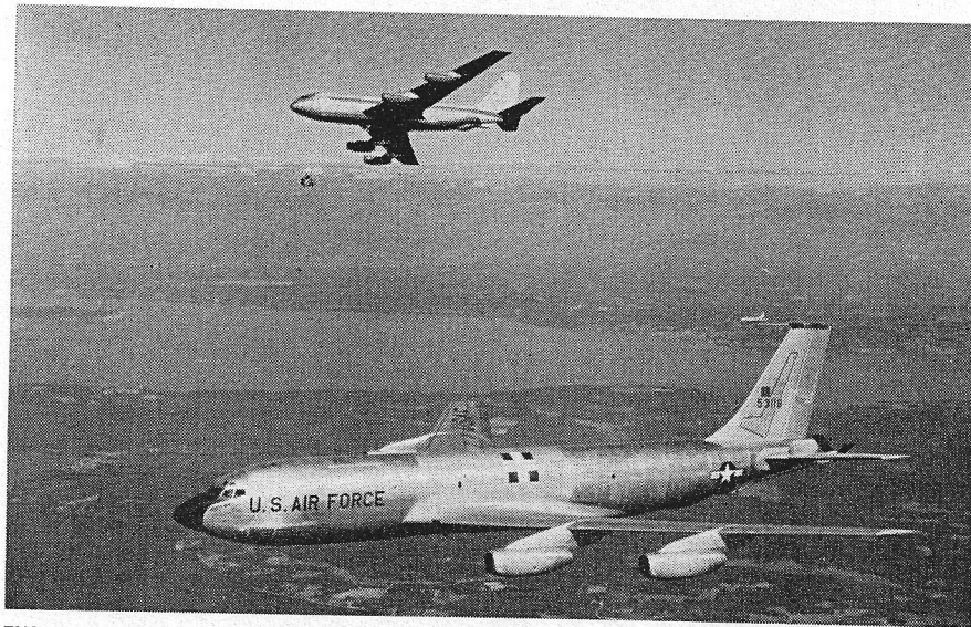
TWO FIRSTS. The Boeing KC-135 Stratotanker "City of Renton" first production model of Strategic Air Command's new tanker transports (nearest the camera) is shown with a sister ship, the Boeing 707 jet transport prototype. This was the initial flight for the tanker. Flying boom equipment for the KC-135 was flight tested earlier on the 707 prototype, America's first jet transport.
