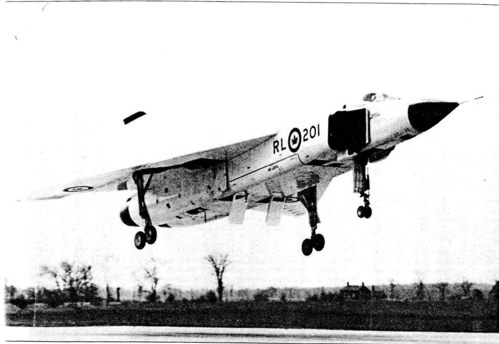
The Arrow with speed brakes extended. (DEPARTMENT OF NATIONAL DEFENCE)
