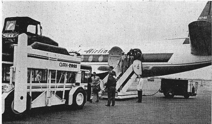
PASSENGER CARRIER. Billed by Canadian Clark Ltd. of St. Thomas, Ont., as the solution to at least one jet age travel problem, the Clark-Ross "Mobile-Cruiser" straddle carrier, shown above is designed to eliminate the costly runway to terminal ground run for jet airliners. Passengers board the pod, which is then picked up by the straddle carrier and transported to the aircraft parked at the end of the runway. The carrier raises the pod to the level of the airliner door. Process is merely reversed for deplaning.
