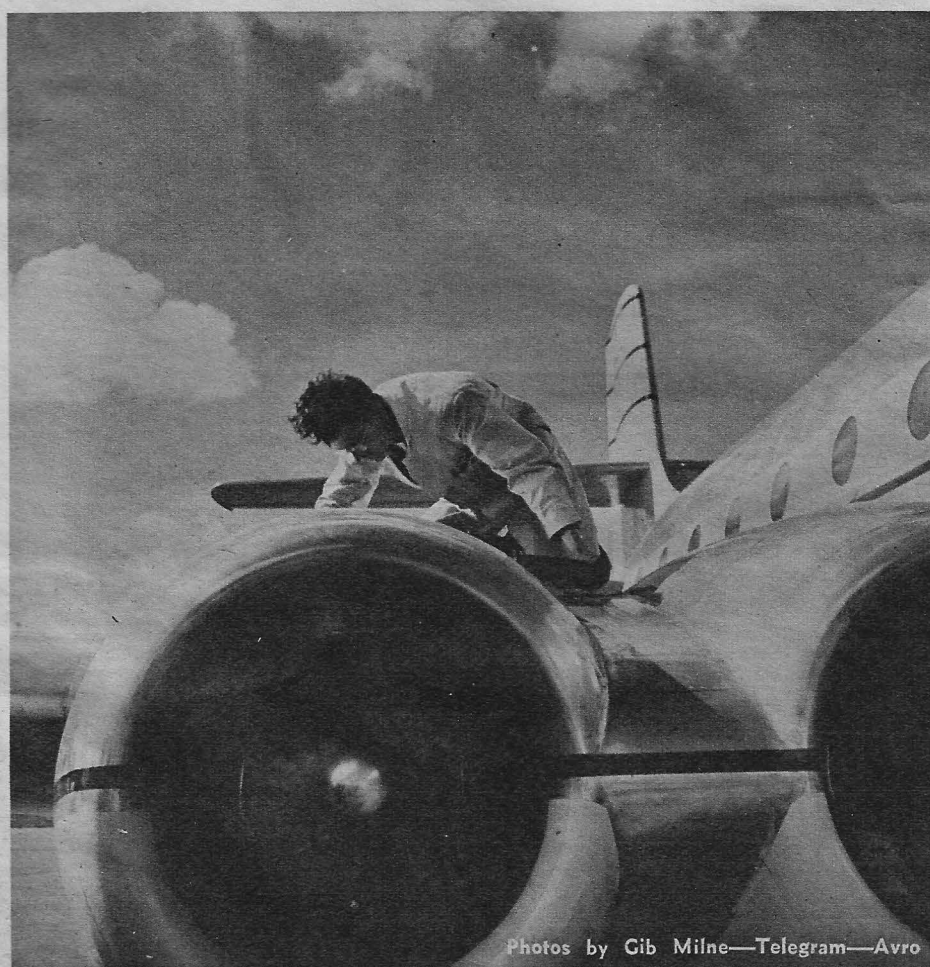
AFTER FLIGHT , a mechanic checks the Rolls Royce Derwent jet engines. During test, Jetliner moved so swiftly it was difficult to keep track of her in sunlight. Speed is 100 mph faster than existing transports.
