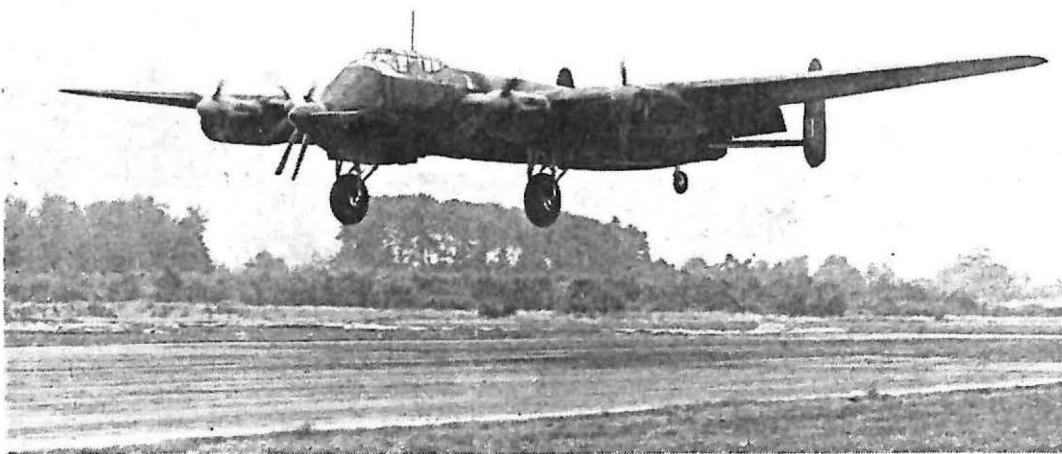
A flying test-bed of more than usual interest, if not beauty—the Napier Nomad-Lincoln, seen arriving at Farnborough on Merlin-power alone.
