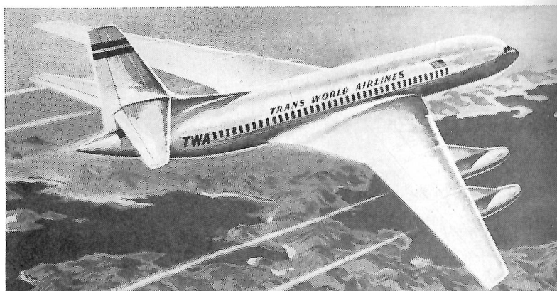
GOLDEN ARROW: Scheduled for delivery to TWA early in 1959, the Convair Golden Arrow medium range jet transport (above), will have a cruising speed of 609 mph and will be powered by four GE J-79/CJ-805 turbojets of approximately 15,000 lb. th. each. The Golden Arrow is ostensibly almost identical to the Skylark 600 announced earlier. Horizontal stabilizer is mounted on the fuselage of the Skylark; Golden Arrow is distinguished by its gold finish.
