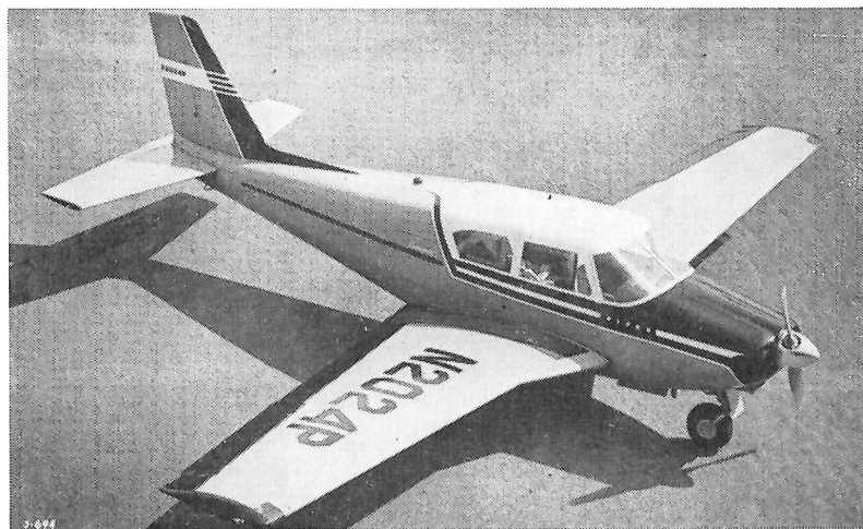
FIRST FLIGHT: The prototype of Piper's new four-place all-metal "high performance business aircraft, the "Comanche", had completed 10 hours flight testing by the end of May. The initial flight tests, using a 180 hp Lycoming engine, indicated that the aircraft equals or exceeds design performance in all respects, according to the manufacturer. Production tooling is underway and deliveries are expected to begin early in 1957. Final choice of powerplant is still to be made.
