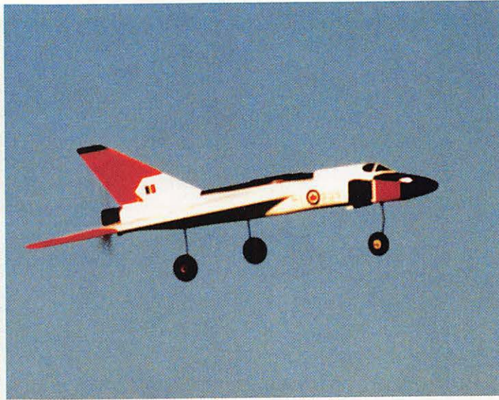
▲ Another low pass for the camera shows the landing gear is out of character, but it can be removed. A bungee launch system works well to get a fast smooth launch.
