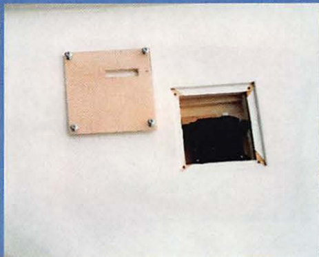
▲ Here you see one of the two elevator servo access hatches that are built into the bottom of the wings.
