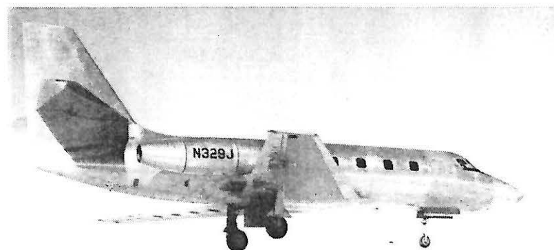
LOCKHEED JETSTAR: Seen above on the ramp, and below in flight for the first time, the Lockheed JetStar presents a study in speed. The 500-550 mph, 10-passenger utility jet transport is at Edwards AFB for flight tests. Pods on rear fuselage contain Bristol Orpheus engines, with take-off thrust totalling 10,000 lbs. The JetStar's 53-foot wing has a 34-degree sweep back on the leading edge.
