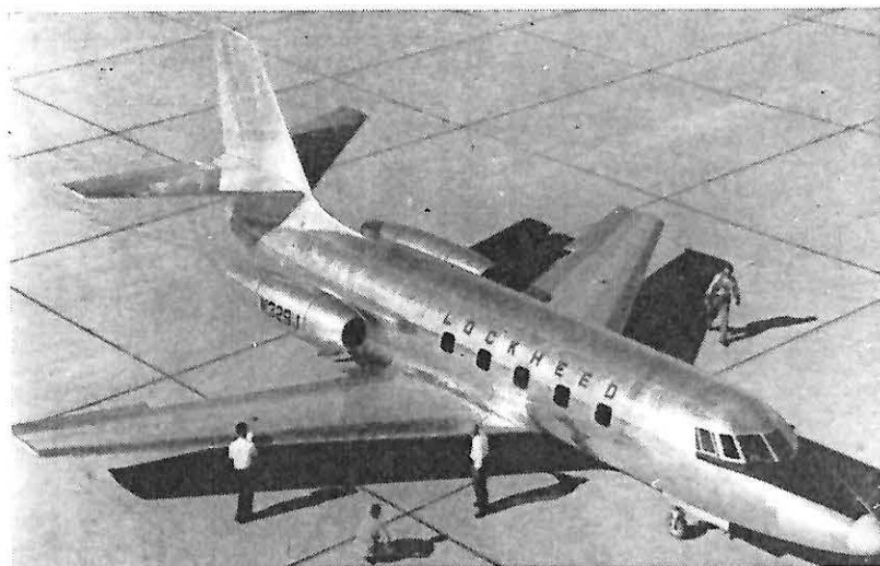
LOCKHEED JETSTAR: Seen above on the ramp, and below in flight for the first time, the Lockheed JetStar presents a study in speed. The 500-550 mph, 10-passenger utility jet transport is at Edwards AFB for flight tests. Pods on rear fuselage contain Bristol Orpheus engines, with take-off thrust totalling 10,000 lbs. The JetStar's 53-foot wing has a 34-degree sweep back on the leading edge.
