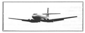
As it happened, with the engines located as close to the fuselage as they were in the four-engined configuration, the 'engine out' handling was so satisfactory that in the cockpit you would hardly be aware of an engine cut as far as yawing was concerned. You could cut a throttle on the plane and, with your feet on the floor, it would go along with a very small adjustment of the trim. Eventually the powered portion of the rudder was locked out as only the manual portion was required.
