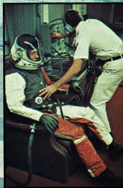
LEFT: Physiological Support Division technician Sgt. Loreli Maslen tests a helmet during preventive maintenance checks. ABOVE: PSD technician Sr. Amn. Douglas Snavelly checks operation of the high altitude pressure suit worn by Maj. Warren Pierce.
