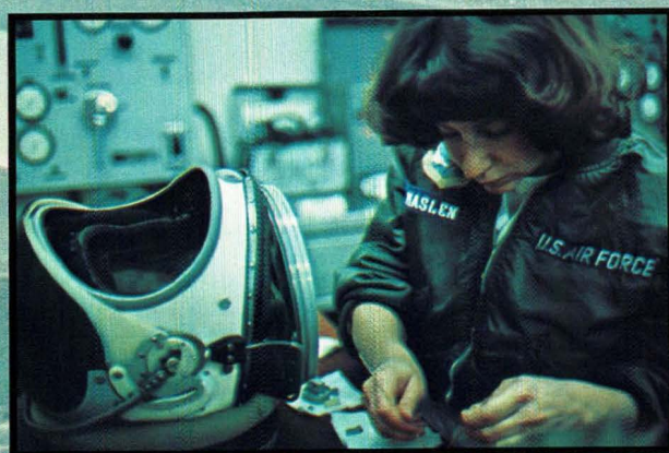
LEFT: Physiological Support Division technician Sgt. Loreli Maslen tests a helmet during preventive maintenance checks. ABOVE: PSD technician Sr. Amn. Douglas Snavelly checks operation of the high altitude pressure suit worn by Maj. Warren Pierce.
