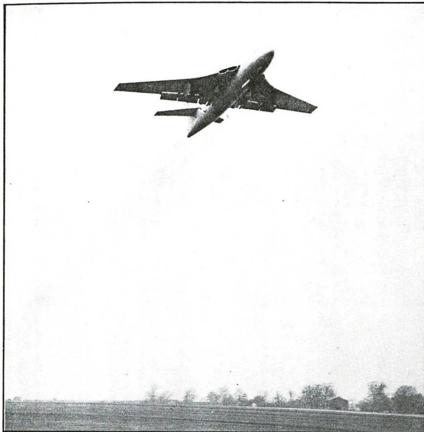
A Vickers Valiant is shown taking off with the assistance of two de Havilland Super Sprite rocket motors, which are contained in jettisonable cannisters.
