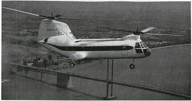
FIRST PICTURE released for publication of the Vertol Model 107, built to carry 25 passengers, or 22 troops. Powered by two turbine engines, the 107 is claimed to have very competitive capacity and speed, plus the reliability of a twin. Prototype is shown flying over the Delaware Memorial Bridge, near Wilmington, U. S. Army has ordered 10 of the Model 107s.
