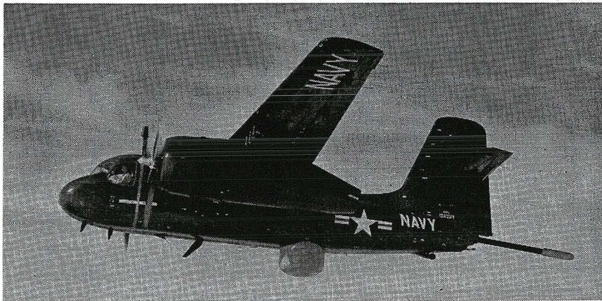
U. S. Navy S2F foreshadows the DH CS2F-1, now being built in Canada for the RCN. Note the extended radome housing and MAD boom, shown here for the first time.
