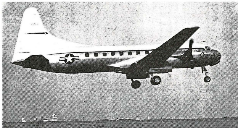
TWO TURBINE TYPES: Above is the Convair YC-131C, taking off on its first flight recently. The YC-131C is the first U.S. military twin-engine turboprop transport and is powered by Allison YT-56 engines, each developing 3,750 hp. Below, the prototype Super Constellation is being used as a flying test bed to test turboprop engine installation to be used on forthcoming Lockheed C-130 military transport. C-130 will also be powered by the T-56, of which it will have four.
