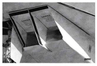
The configuration of the air intakes to the engines in order to provide adequate engine efficiency at all speeds was also a special problem; this required an advanced system of variable-geometry ramps and air spill doors, similar to that we were to use on the Mk. 3 Arrow.
