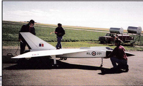
Arrow 2000 Project's 1/5th scale flight test model.
