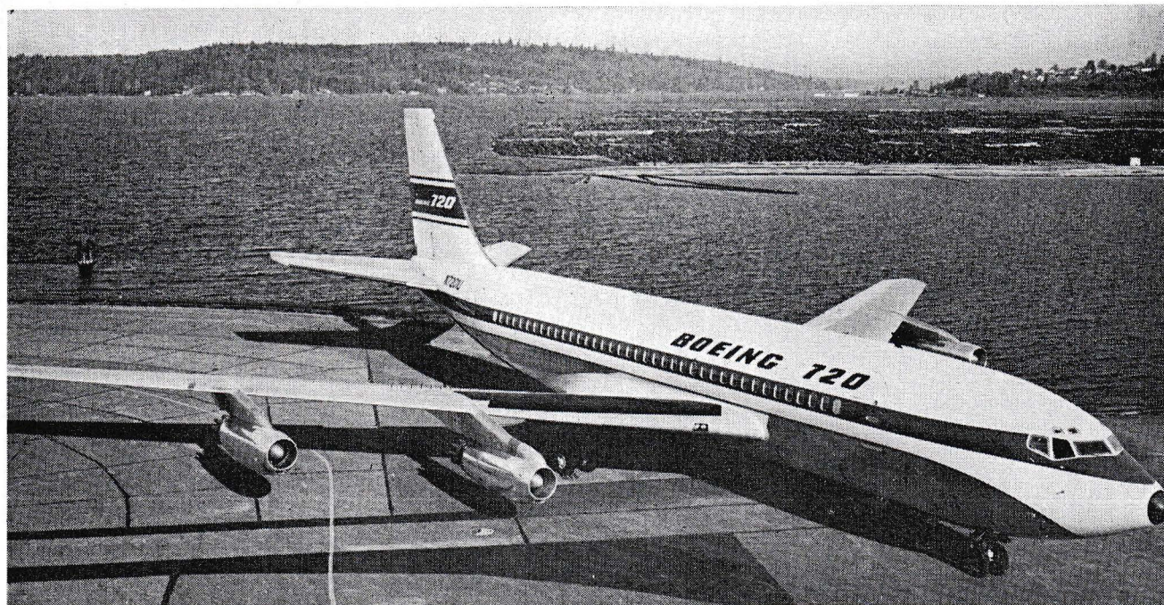
MEDIUM RANGE JET. Boeing rolled out the first 720 medium range jetliner last month. American Airlines has ordered 25 of the shortened and lightened version of the 707, and Irish Air Lines, three. 720 will cruise at over 600 mph, carry up to 150.
