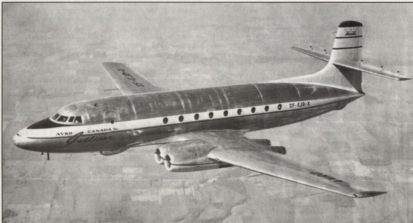
Below: Another inflight photo from the air-to-air soiree shown on top of facing page shows the jetliner's amazingly clean lines. Notice cabin air intake scoop on lower fuselage, just below the single passenger door located forward of the left wing.
