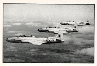
The T-33AN Silver Stars shown above differ externally to no appreciable defrom the original Lockheed T-33A jet trainer illustrated in the three-view at right. The Canadairbuilt Silver Star has, of course, the Rolls-Royce Nene 10 as a powerplant current Lockheedbuilt T-33A's are fitted with Allison J-33's. It will be noted that the cockpit canopy on the Canadair model is a single sheet of clearview plastic, unbraced except by the outer frame; earlier U.S. versions, however, have a stiffener in
