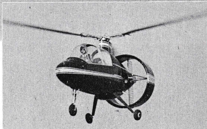
Lufthansa airline forsee's Mach 3 canard type transport like model (above). Four powerplants of 40,000-lb thrust each suspended under aft delta wing. Span 98-ft. length 203-ft; gross weight 400,000-lb; 140 passengers. Second prototype of Canada's Avian 2/180 "Gyroplane" (right) equipped with mechanical rotor spin-up system undergoes air-worthiness test. Target price for production craft, $15,000. Two place; 180-hp Lycoming power.
