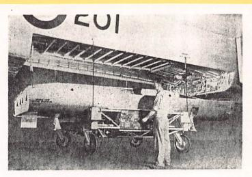
ARMAMENT PACK is designed for fast replacement. Several different missile weapon packs can be used interchangeably. The pack is lifted into place by a self-hoisting mobile support carriage (which also serves as a transport dolly) and is secured flush with the underside of the fuselage at four connection points. Estimated size of armament bay is 16x9x21/2 ft. Arrows show hoist point.
