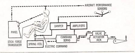
AUTOMATIC FLIGHT CONTROL system includes damping to augment longitudinal dynamic stability at altitudes over 40,000 ft for weapon launching. System also augments lateral static and dynamic stability at high altitudes and speeds for basic controllability. Emergency damping system is duplicated in the yaw axis.
