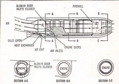
CF-105 was to be powered by two Orenda Iroquois engines with integral after-burners. Over Mach 0.5, ram air opens intake gills near compressor to bypass cooling air around engine. This also reduces spillage at high speeds. Result is near-optimum performance at all speeds despite fixed geometry intake.
