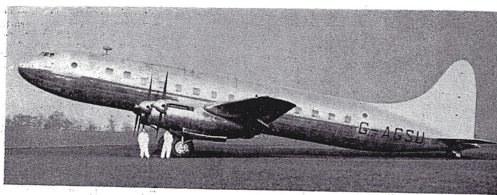
The Avro Tudor II pictured here has been test flown in England and will be made in the Malton plant of A. V. Roe (Canada) Ltd. The 320-ft. span airliner can carry 60 people 1,850 miles at 230 m.p.h., or as a freighter, has a capacity of nine British tons, a range of 1,100 miles at 200 m.p.h.
