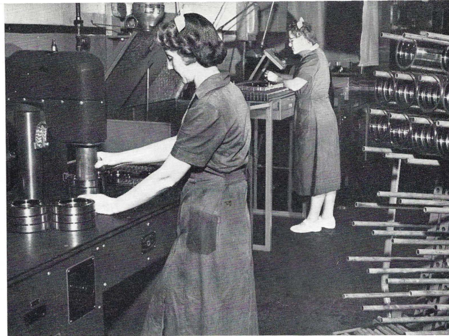
Magnafluxing is important checking operation. Rings are magnetized in instrument at left, then immersed in bath containing fluid in which minute particles of magnetic compound are suspended. These particles cluster to any defect which is then revealed under magnifying lens to the operator at right.
