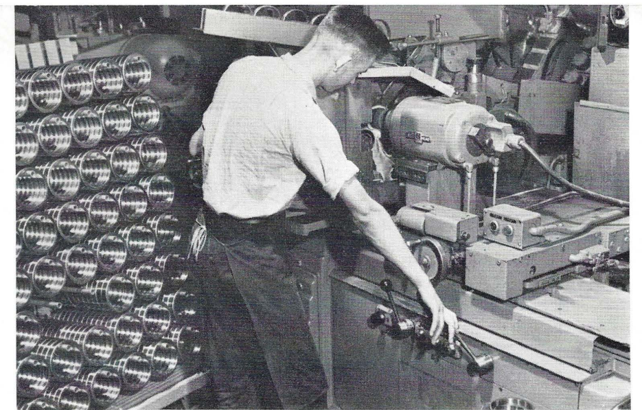
Raceway of roller bearing is ground in Heald Size Matic Internal Grinder. Workpiece is held by a set of rollers against a rotating backing plate thus assuring almost perfect concentricity between the outside die and the raceway.
