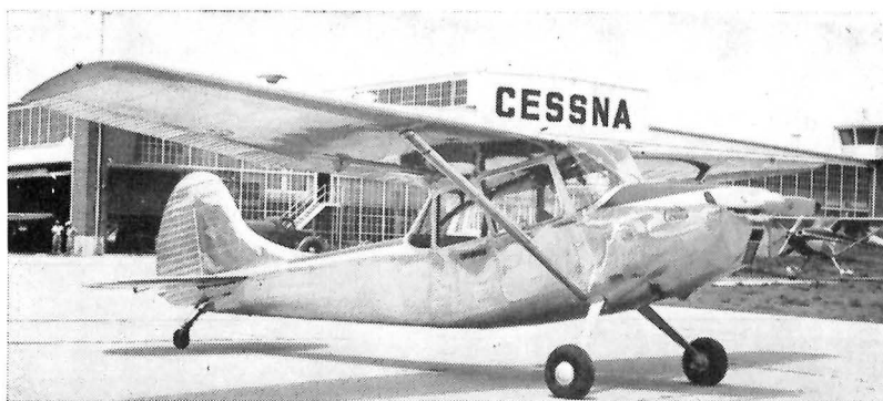
THE WINNER: Cessna Aircraft Company's Model 305 liaison plane was recently named winner of the U.S. Army Field Forces competition to choose an aircraft suitable for observation-reconnaissance. The military designation of the machine will be the L-19. It is powered by a 190 hp Continental engine and has a range of speeds from 43 knots up. Normal cruise is 90 knots. The airplane carries 42 gallons of fuel and has a gross weight of 2,100 lbs.
