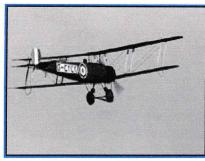
prevented the plane from dropping dramatically when power was reduced, and the "forgiving" quality of its controls were ideal for training. So too was the skid that could be outfitted under the nose, designed to prevent tipping during landing.
