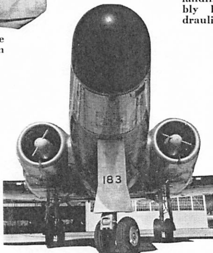
ABOVE: CF-100 plastic nose radome by Brunswick-Balke-Collender Company.
