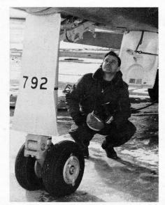
PRE FLIGHT CHECK of 792 last CF-100 to roll off Avro's production line is made by Chief Production Pilot Chris Pike prior to taking the airplane into the air for the first time recently for a production flight test. All pilots personally check each airplane visually from the ground before climbing into the cockpit for further checks before taxiing out to take off.
