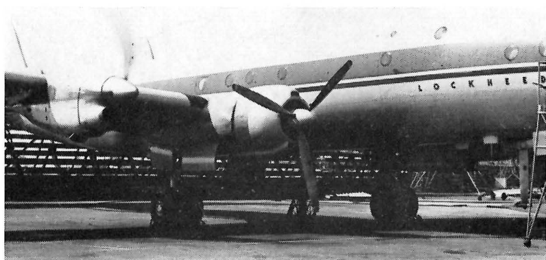
TWO TURBINE TYPES: Above is the Convair YC-131C, taking off on its first flight recently. The YC-131C is the first U.S. military twin-engine turboprop transport and is powered by Allison YT-56 engines, each developing 3,750 hp. Below, the prototype Super Constellation is being used as a flying test bed to test turboprop engine installation to be used on forthcoming Lockheed C-130 military transport. C-130 will also be powered by the T-56, of which it will have four.
